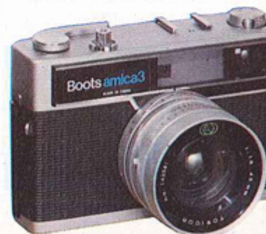
Boots Amica 3 Camera £38-17-0 Outstanding CdS 35 mm. camera. The Amica 3 can be used both fully automatically or on manual over-ride. It has fast f/1.8 six-element lens, coupled CdS meter, built-in rangefinder, ten-speed shutter, delayed action facility and is fully synchronised for flash. The meter is within the lens mount for automatic filter compensation. Ever Ready Case 79/- Japan
